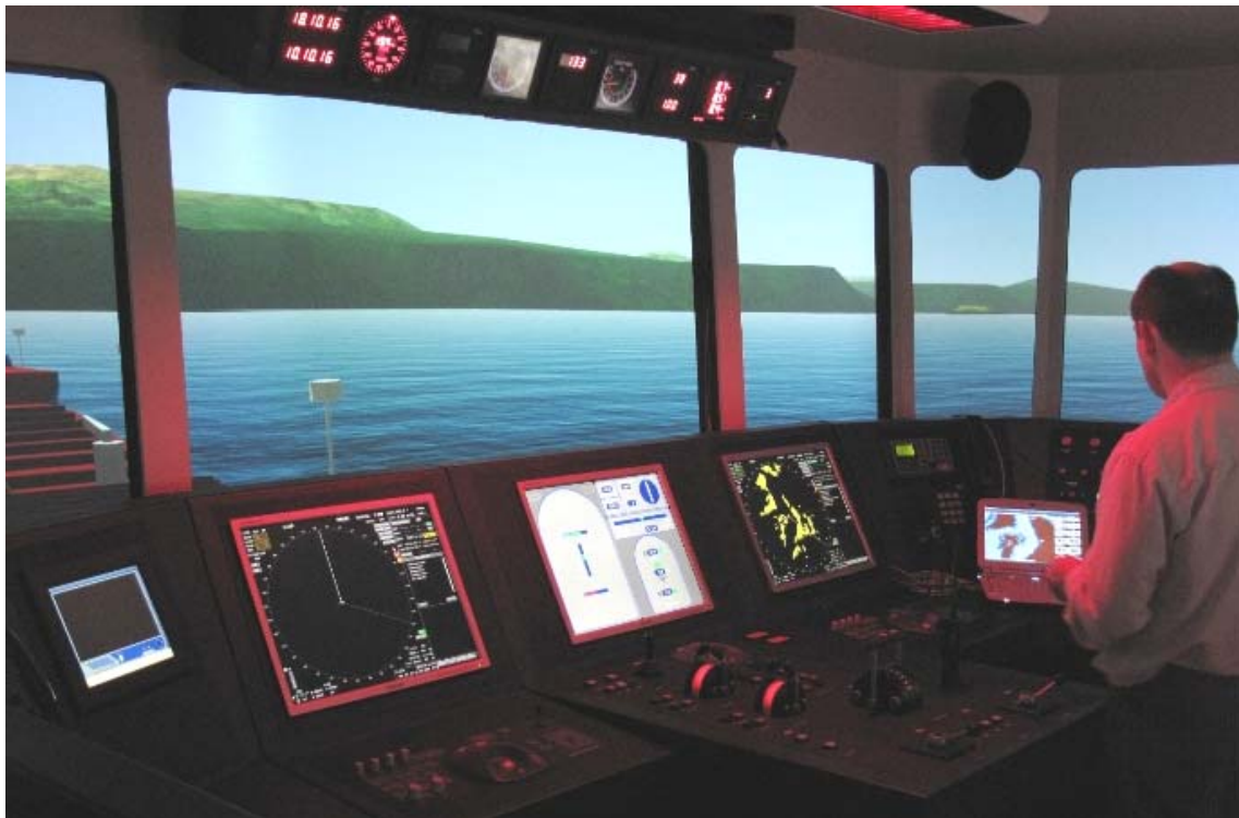
Figure 3-6 View from the simulator bridge showing the navigational equipment and control handles for the engine and rudder.
