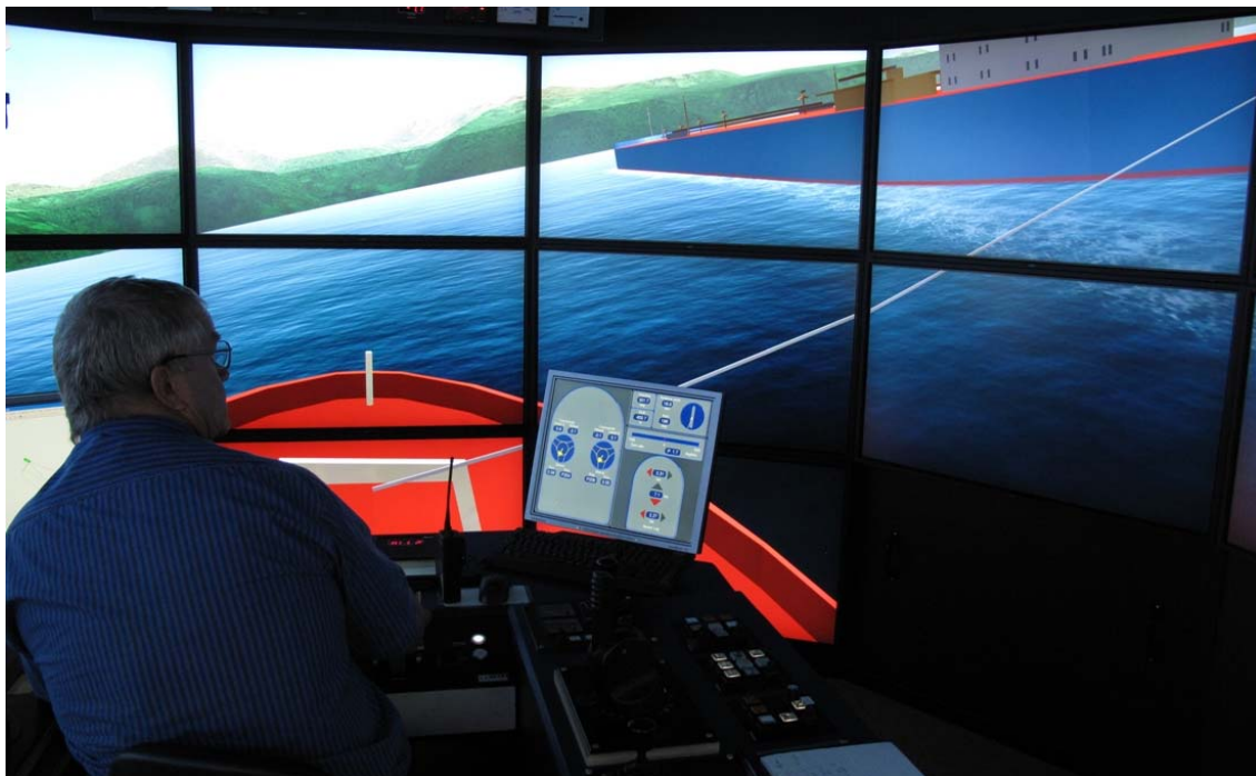
Figure 3-11: A tug master towing in indirect escort mode on tug bridge "H" - a 360 degree field of view state of the art simulator.
