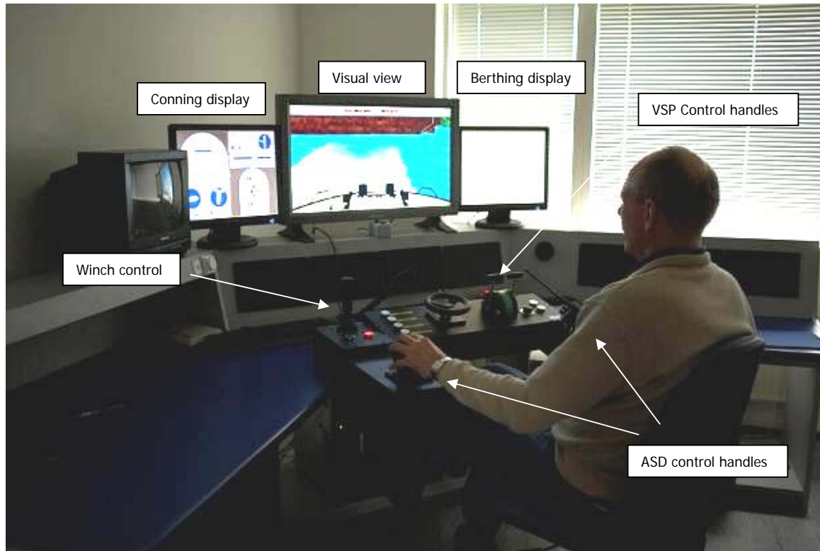
Figure 5.5 Auxiliary tug control cubicles
