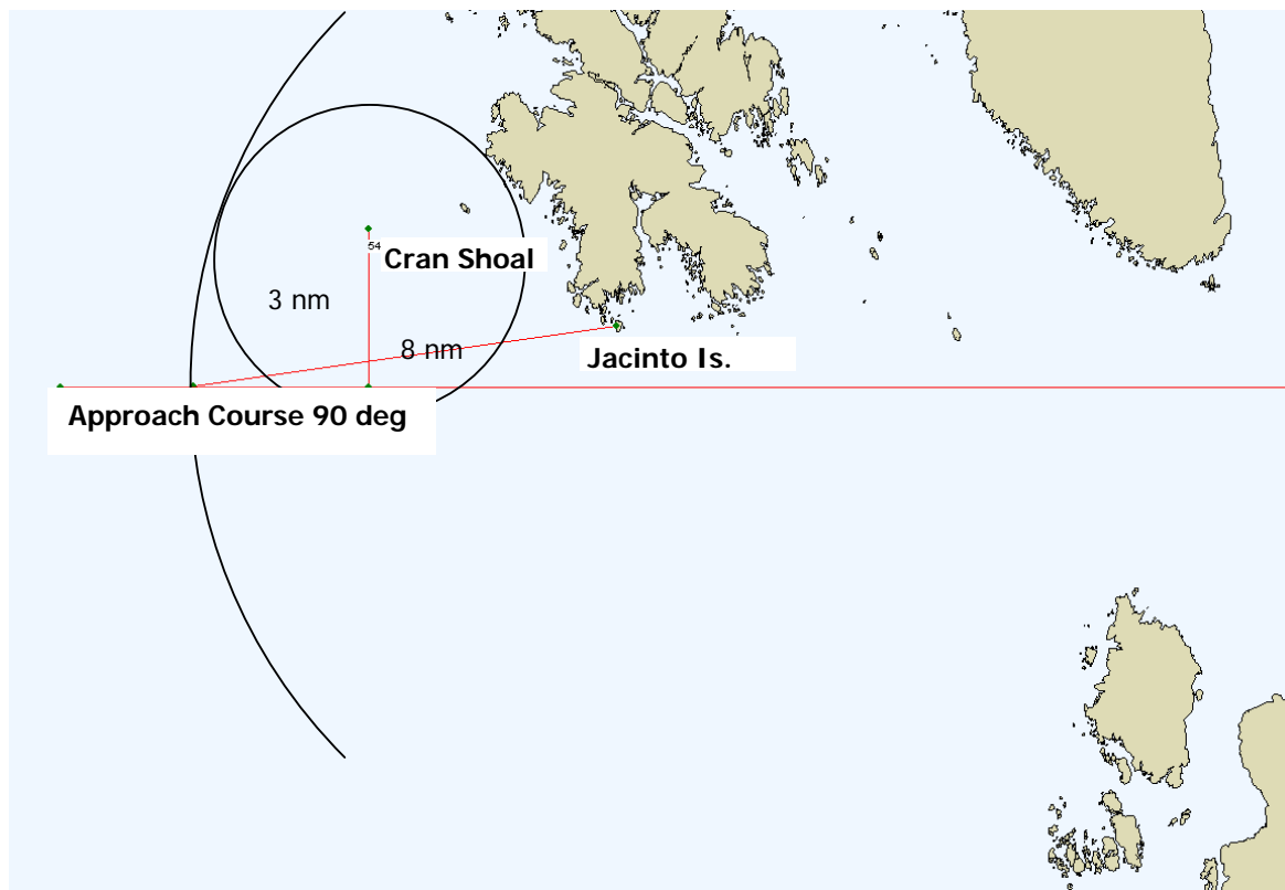
Figure 6.7 Definition of Point Of No Return (P.O.N.R.)
