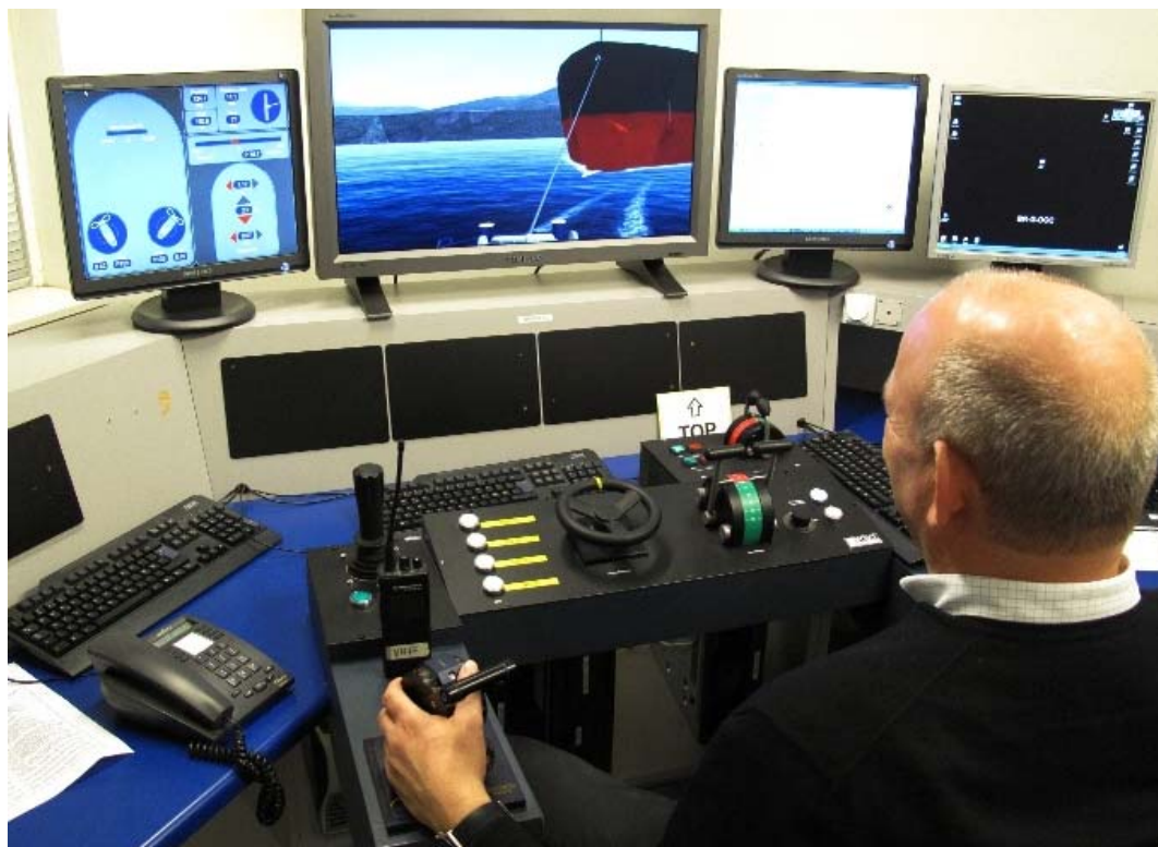
Figure 3-7 A tug master in front of one of the tug simulators used in the study. Note: On the visual view you can see the tow line that is connected from the tug's bow to the tanker's bow. This photo was taken in connection with a berthing manoeuvre close to the oil terminal.
