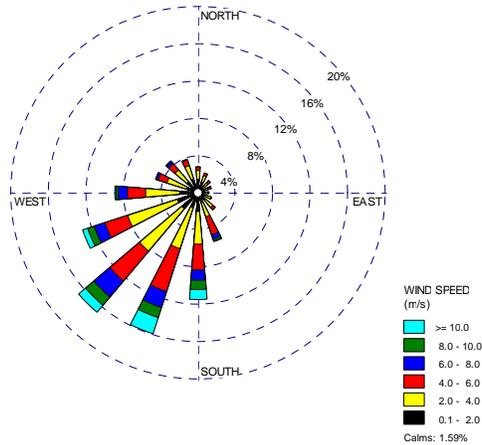
**Figure F-7 Comparison of Modelled Surface Winds (2002) at Four Locations (B, C, D and E in Figure E-6)**
