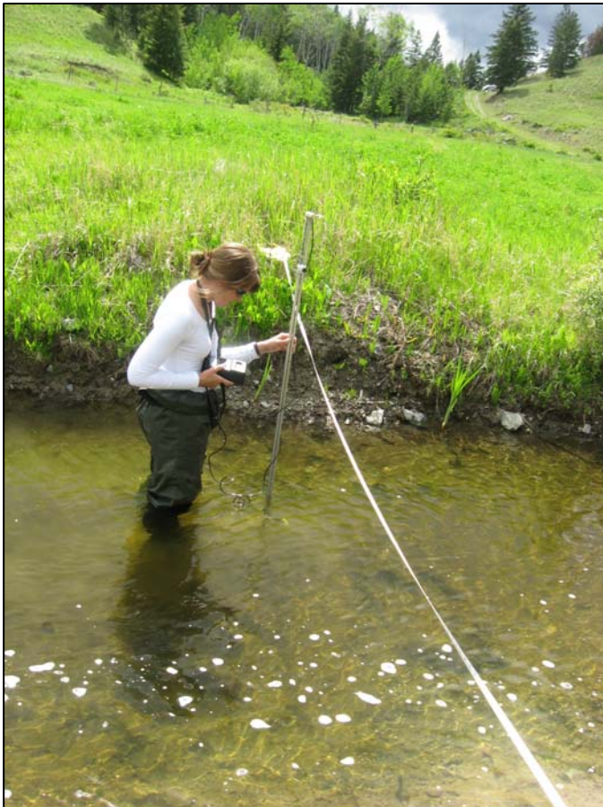
PHOTO A6 – JACSEEP Velocity-Area Discharge Measurement
