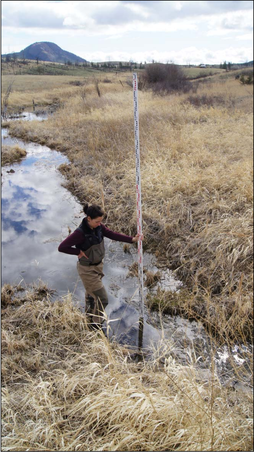
PHOTO A11 – TSFINF Cross Section Survey of Secondary Channel
