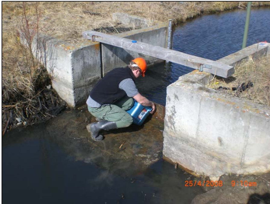
PHOTO A7 – JACSEEP Volumetric Discharge Measurement
